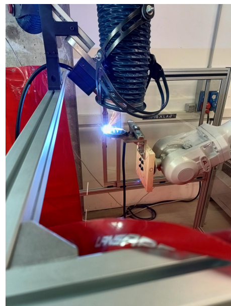
Fig. 23 – Robotized WAAM process in action
