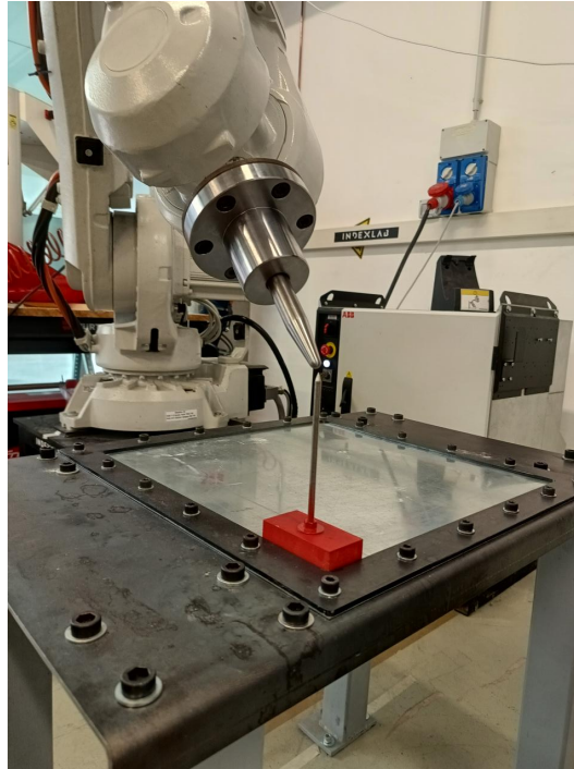
Fig. 49 – Calibration for the incremental sheet forming process
