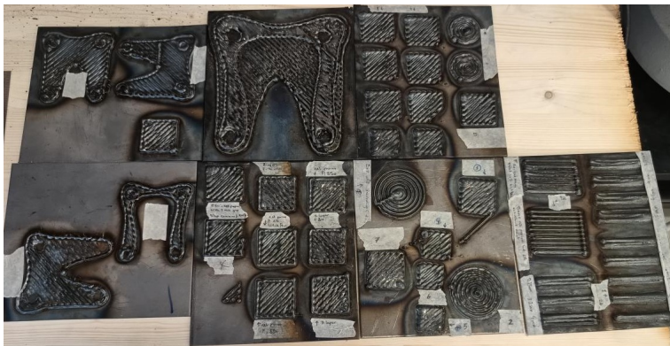
Fig. 20 – WAAM WASP dispositive printed pieces
