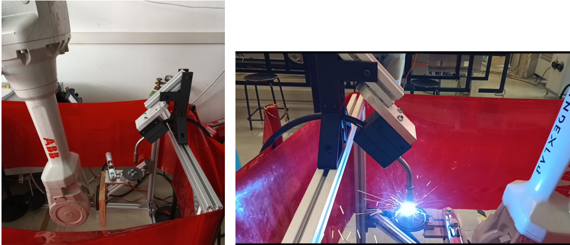
Fig. 21 – First setup of robotized WAAM
