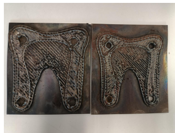
Fig. 20 – WAAM WASP dispositive printed pieces
