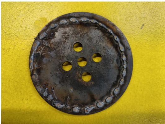
Fig. 25 – No gas test
